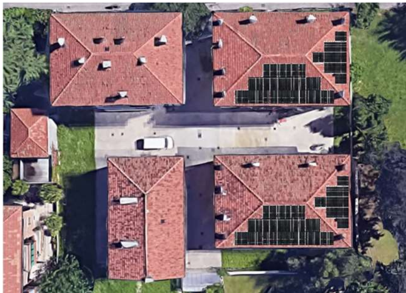
Figure 60 – On-roof PV plant on the social house blocks
